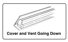
10. As the ventilator intake is lowered, the cover will return to its position covering the ventilator.
